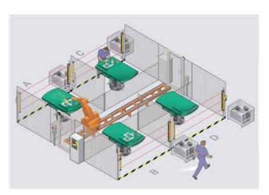
All safety components in each of the two areas are attached to a Flexi Soft safety controller station which are in turn connected with one another over Flexi Link. If there is a complete stop of the robot, the dangerous action of the turntable will also stop. If one area of the machine has stopped, the robot can work in the other area until the stopped section is brought back online. The switch off signal is sent directly from the Flexi Soft safety controller. After a complete stop, the
