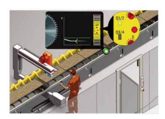
worker can now activate Safety Limited Speed (SLS) in order to service the sawline through use of the E100 enabling switch. The sawblade is only allowed to run if its speed stays within the set limit and the enabling switch remains pressed. If at malfunction the speed limit is exceeded, the drive will be switched off by the Speed Monitor MOC3SA to avoid injury. In order to acheive safety limited speed, the Speed Monitor MOC3SA constantly compares the speed of the saw
